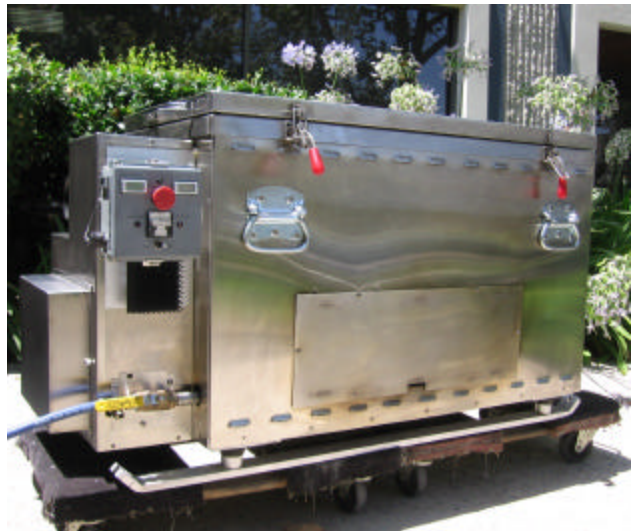
Figure 8. Self-powered tray ration heater
