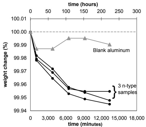
FIGURE 7. Weight Loss of N-Type at 255 °C.
