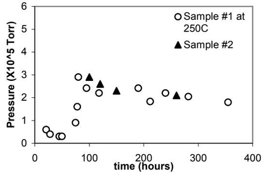
FIGURE 6. Vacuum Chamber Pressure vs. Time Curve With and Without the RTG Insulation.
