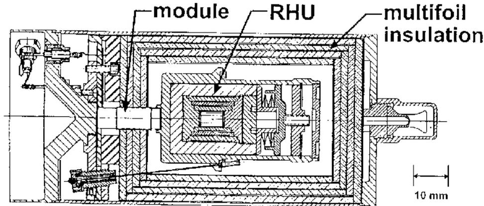
FIGURE 1. Milliwatt Radioisotope Power Supply
