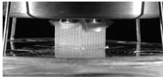
FIGURE 2. Fuel Capsule Mounted on Module with a Layer of Kapton® between the Module-Fuel Capsule Interface.
