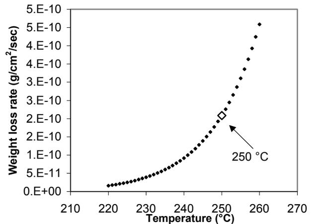
FIGURE 10. Te<sub>2</sub> Weight Loss Rate as Function of Temperature.
