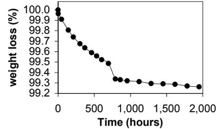
**FIGURE 8.** WeightLoss of P-Type @ 255° C
