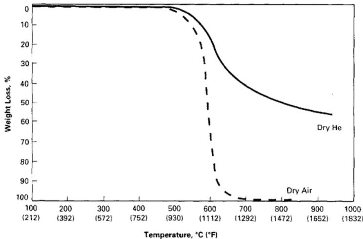
FIGURE 3. Kapton® Weight Loss in Helium and Dry Air.
