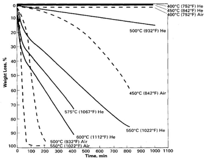
FIGURE 5. Kapton® Weight Loss at 250 °C.
