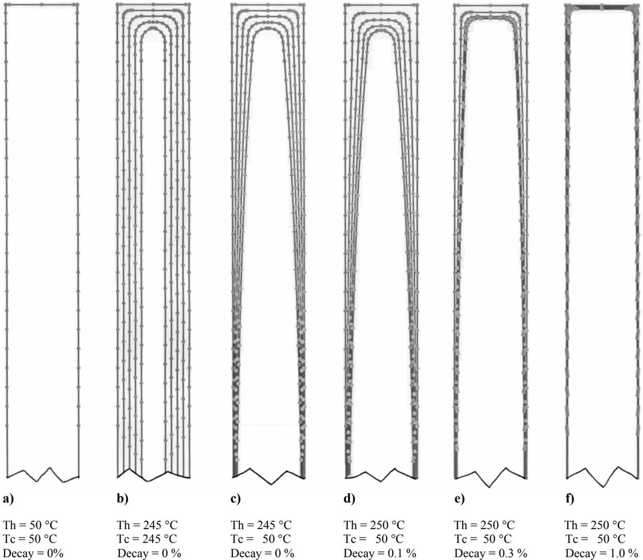
**FIGURE 9.** 2-D Surface Profile of Leg Hot Side as a Function of Initial  $T_{hot}$ ,  $T_{cold}$ , and RHU Power Decay Rate. Scale 50 X 1.
